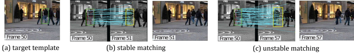
Figure 4.7 – The appearance of the target is represented by a template in a video frame (a). In figure (b), a set of sampled points \{\mathbf{u}_i\} inside the target in frame 50 matches to a set of points \{\mathbf{v}_i\} in the frame 51. The optical flow is computed from densely sampled points inside the target template to a new frame. The quality of the flow is used as a cue to make the decision: (b) an example of stable prediction, meanwhile the divergence of matching point caused by the unstable prediction (c). The yellow box is the predicted location of the target. [229]
