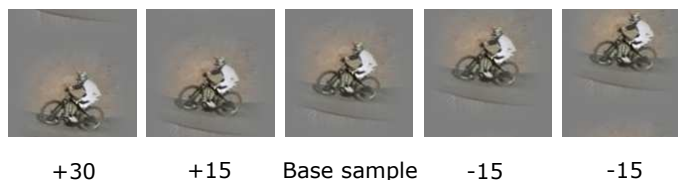
Figure 2.11 – Example of vertical cyclic shifts of a base sample. The formulation in the Fourier domain allows the tracker to be trained with all possible cyclic shifts of a base sample, both vertical and horizontal, without iterating them explicitly. Artifacts from the wrapped-around edges can be seen (top of the left-most image), but are mitigated by the cosine window and padding. [102]
