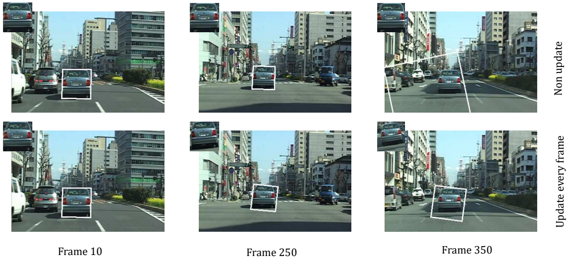
Figure 3.5 – An example of drift problem in [153]. The first row illustrates the tracker is failing to track the car after not updating any new target’s appearance at all. The second row shows the templates being updated every frame which leads to the undesirable updates resulting in drift problem.
